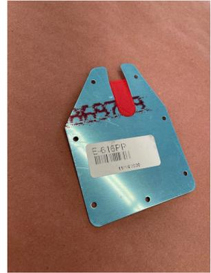
2-Drill the 4 holes through the Drill Guide Template with a 3/32 (#40) drill. Remove the template and now drill the holes with a #28 drill.
