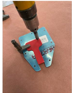
3- Dimple the 4 holes. Make sure the dimples are on the same side (if you already have completed this step in the plans) as the attachment holes of the plate.
