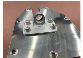
4- Check the fit by inserting the 4 screws. **Do not use a powered screwdriver!** If any screws are not going in with a hand screwdriver, use a #6-32 tap and "clean" the hole out. Don't force it. Not nice :)
